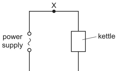
If too much current flows, a component connected at X automatically disconnects the power supply.
